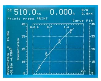
Suspect standards may be observed by inspection of the screen display and either deleted or substituted by a replicate standard.
