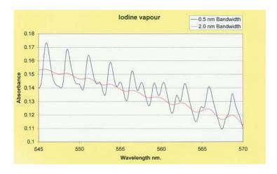
Also shown here is the spectrum of iodine vapour near 560nm.
